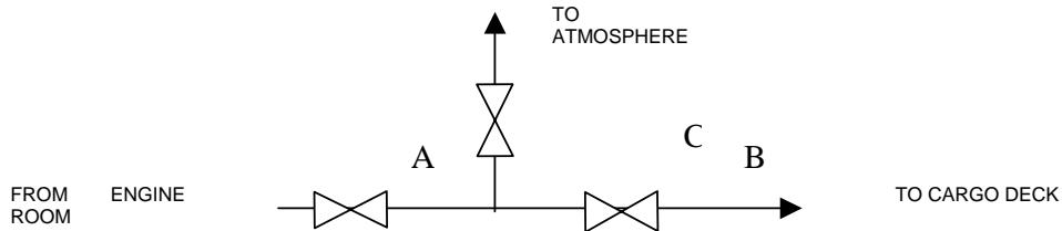
Referring to the above diagram, "A" & "B" are the in-line non-return valves. "C" is a valve on the venting line, which could be pneumatically operated. This valve is linked to the IG generator. This valve closes when the plant is operational and opens when the plant is stopped.
