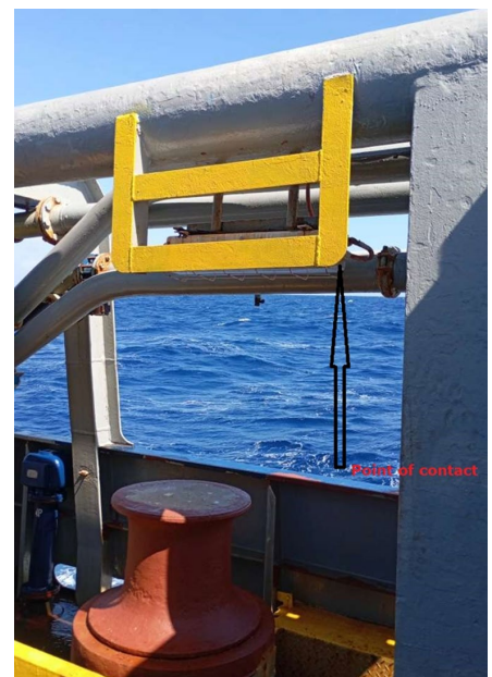
Deck light guard
