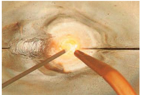
Figure 8. Backhand welding technique.
