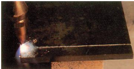
Figure 12. Starting a cut.
