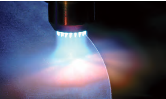
Figure 9. The application of preheat gases.
