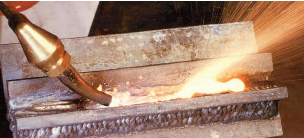
Figure 14. Oxy-acetylene gouging application
